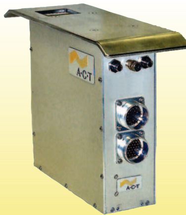
Figure 3. The BXR-1 Backscatter Sensor from Automation and Control Technology Inc. uses multiple solid-state detectors and a cold-cathode X-ray source to measure thickness safely, accurately, and economically.
